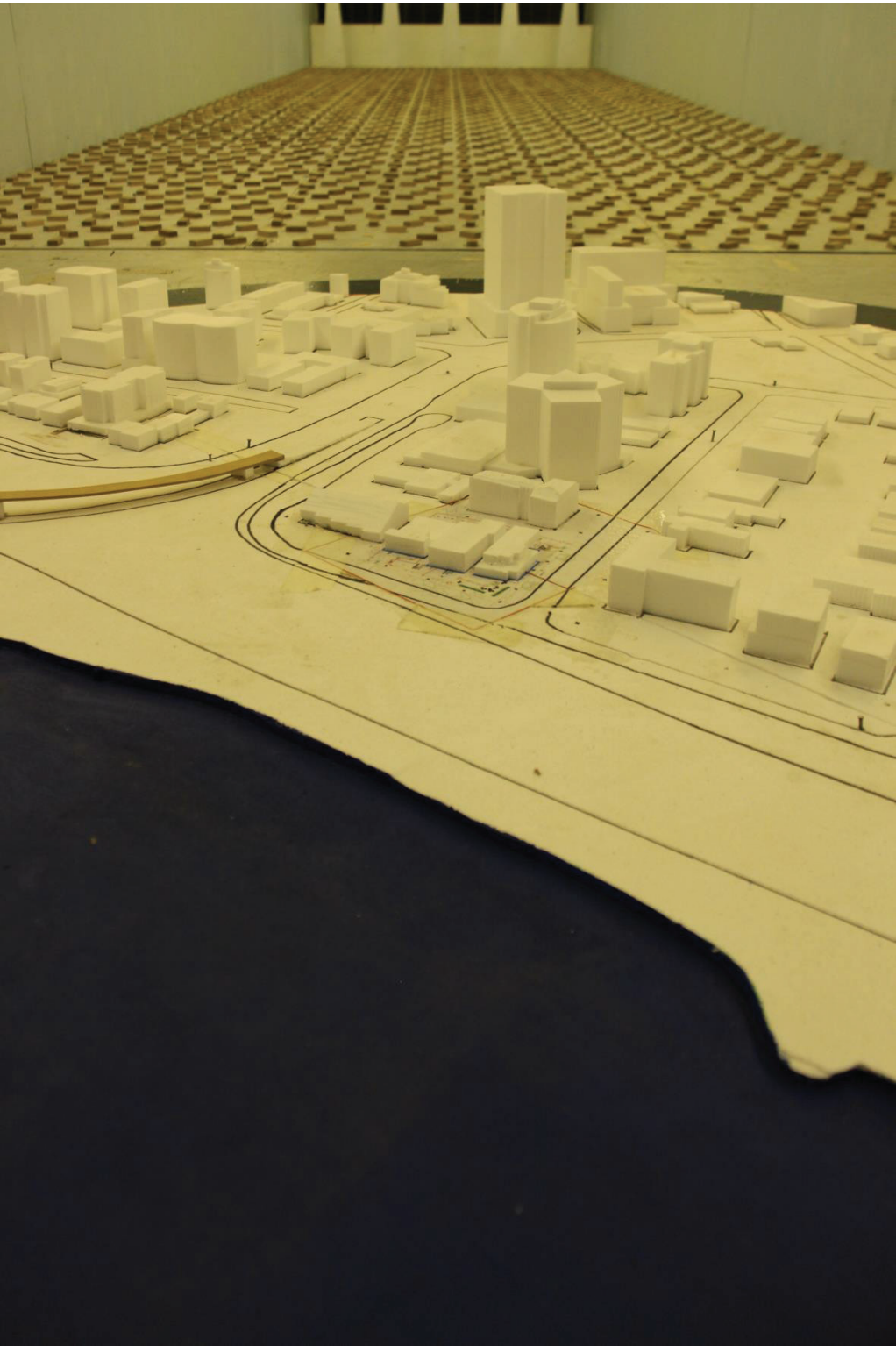
Figure 2f: Photograph of the Wind Tunnel Model - Existing Scenario (view from the south-west)
