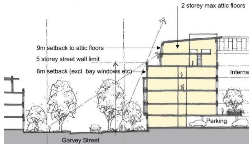
Figure 2: Cross-section of potential development showing heights and street setback
