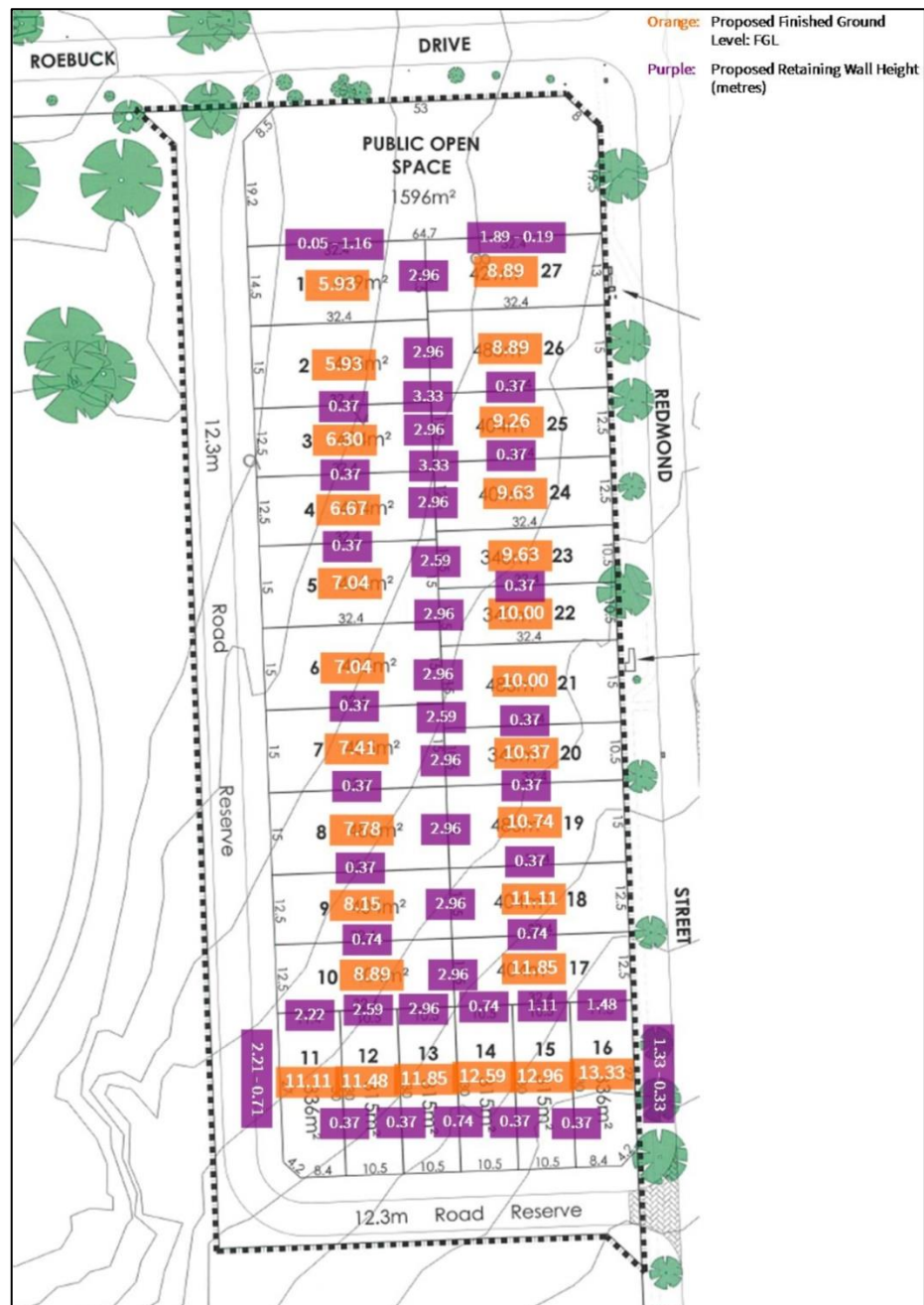
Figure 4 Proposed Finished Ground Levels and the Height of the Proposed Retaining Walls
