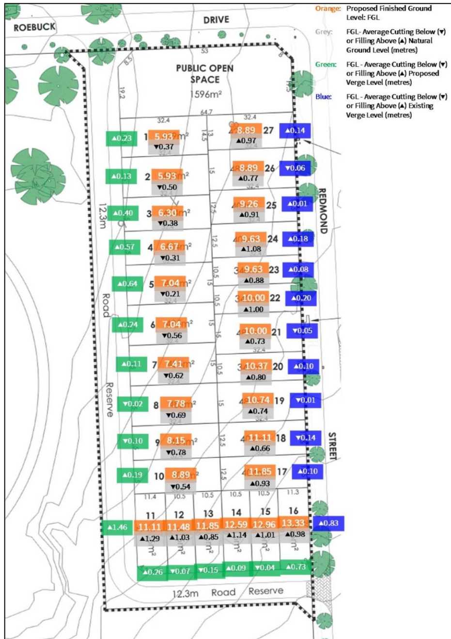
Figure 3 Proposed Finished Ground Levels and the Variation to the 'Equal Cut and Fill' Calculation
