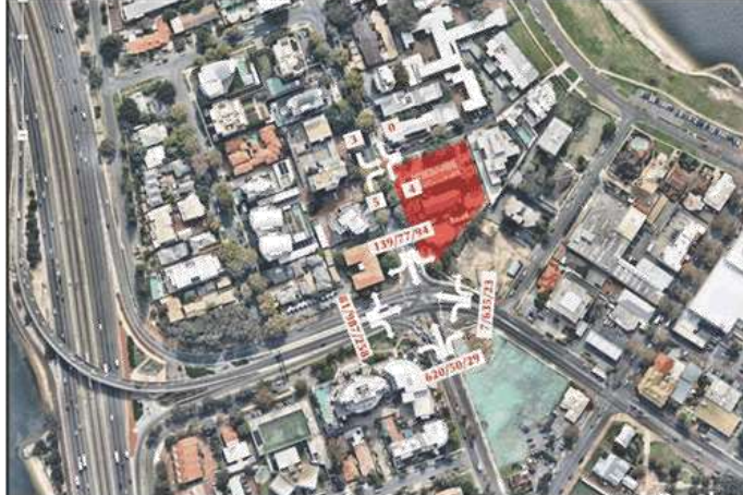
Figure 8. Existing traffic flows at local intersections (survey results + SCATS data) – weekday PM peak hour
