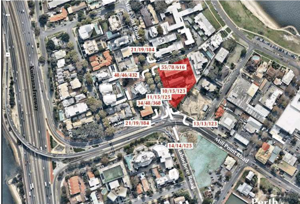
Figure 6: Estimated traffic flows from the proposed development – weekday AM peak hour/PM peak hour/daily traffic
