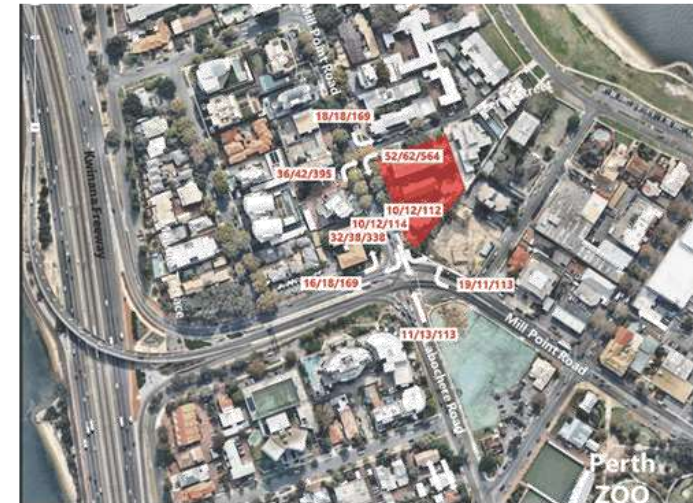
Figure 6: Estimated traffic flows from the proposed development – weekday AM peak hour/PM peak hour/daily traffic
