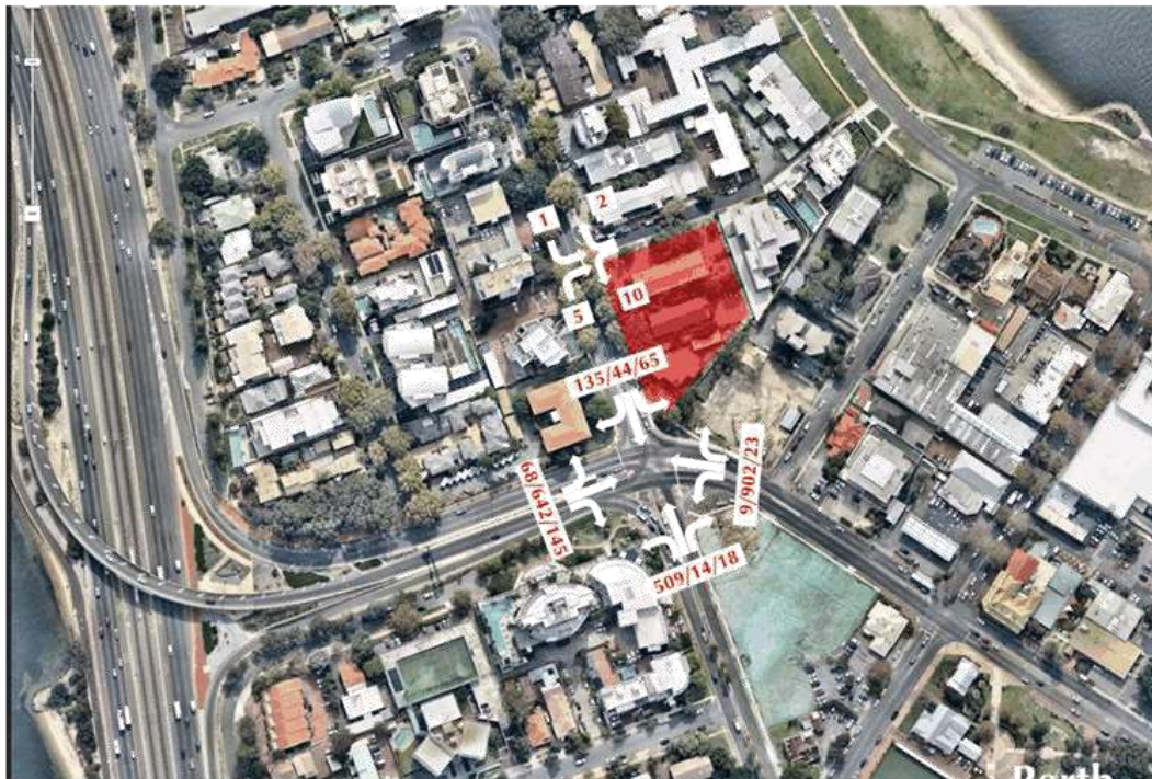
Figure 7. Existing traffic flows at the local intersections (survey results + SCATS data) – weekday AM peak hour
