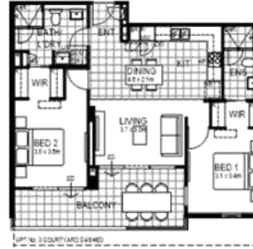
APT. TYPE B 2 BED / 2 BATH APT No's. 9, 10, 17, 24, 31, 38 APT. AREA 76m 2 BALC. AREA 13m 2 C/YARD. AREA FOR APT. 3, 22m 2
