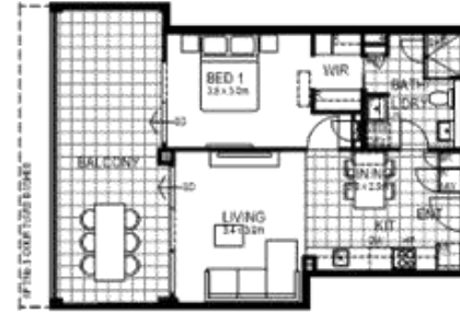
APT. TYPE A1 1 BED / 1 BATH APT No's: 5, 12, 19, 26, 33, 40. APT. AREA: 53m 2 BALC. AREA: 22m 2 C/YARD. AREA FOR APT. 5: 29m 2
