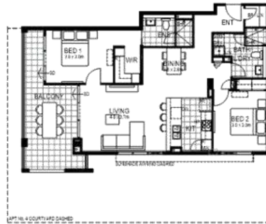
APT. TYPE C1 2 BED / 2 BATH APT No's: 4, 11, 18, 25, 32, 39. APT. AREA: 90m 2 BALC. AREA: 17m 2 C/YARD. AREA FOR APT. 4: 77m 2
