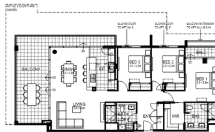
APT. TYPE D 3 BED / 2 BATH APT No's: 6, 13, 20, 27, 34, 41. APT. AREA: 117m 2 BALC. AREA: 31m 2 BALC. AREA FOR APTS 13, 41: 32m 2 C/YARD. AREA FOR APT. 6: 83m 2
