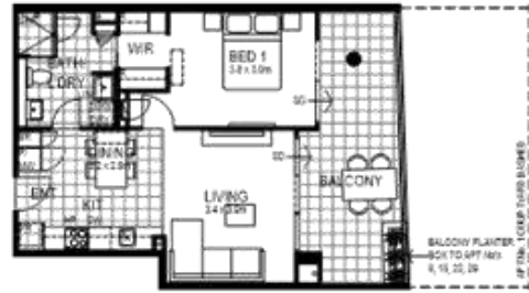
APT. TYPE A 1 BED / 1 BATH APT No's: 1, 8, 15, 22, 29, 36. APT. AREA: 52m 2 BALC. AREA: 15m 2 C/YARD. AREA FOR APT. 1: 40m 2
