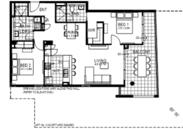
APT. TYPE C 2 BED / 2 BATH APT No's: 2, 9, 16, 23, 30, 37. APT. AREA: 68m 2 BALC. AREA: 17m 2 C/YARD. AREA FOR APT. 2: 94m 2
