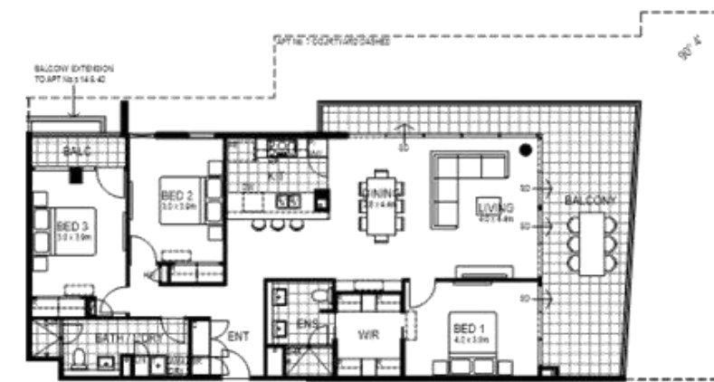
APT. TYPE E 3 BED / 2 BATH APT No's: 7, 14, 21, 28, 35, 42. APT. AREA: 122m 2 BALC. AREA: 30m 2 BALC. AREA FOR APTS 14, 42: 33m 2 C/YARD. AREA FOR APT. 7: 104m 2
