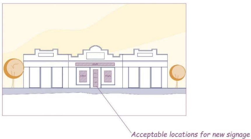
Diagram 1 - New signage shall be located such that it does not obscure original or significant detailing (awnings, shop windows and doors).
