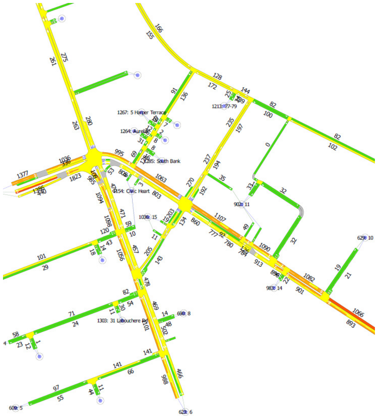
Figure 8 2021 PM Link Volume Plot (vehicles) – Committed Developments Only (Excluding 88 Mill Point Road)
