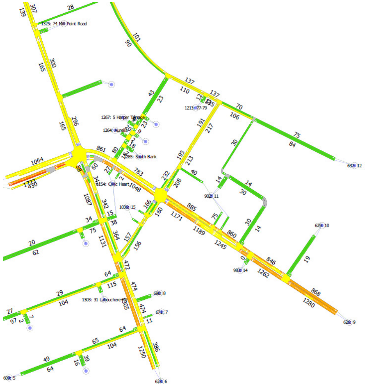
Figure 4 2021 AM Link Volume Plot (vehicles) – Committed Developments Only (Excluding 88 Mill Point Road)
