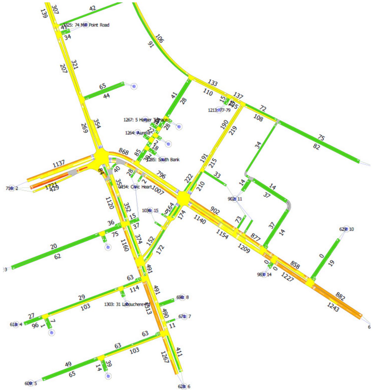
Figure 4 2021 AM Link Volume Plot (vehicles) – Committed Developments with 74 and 88 Mill Point Road
