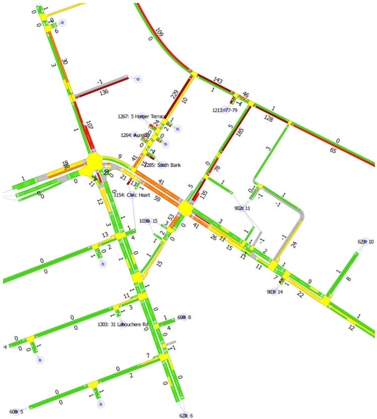
Figure 6 2021 PM Link Delay Plot (seconds) – Committed Developments with 74 and 88 Mill Point Road
