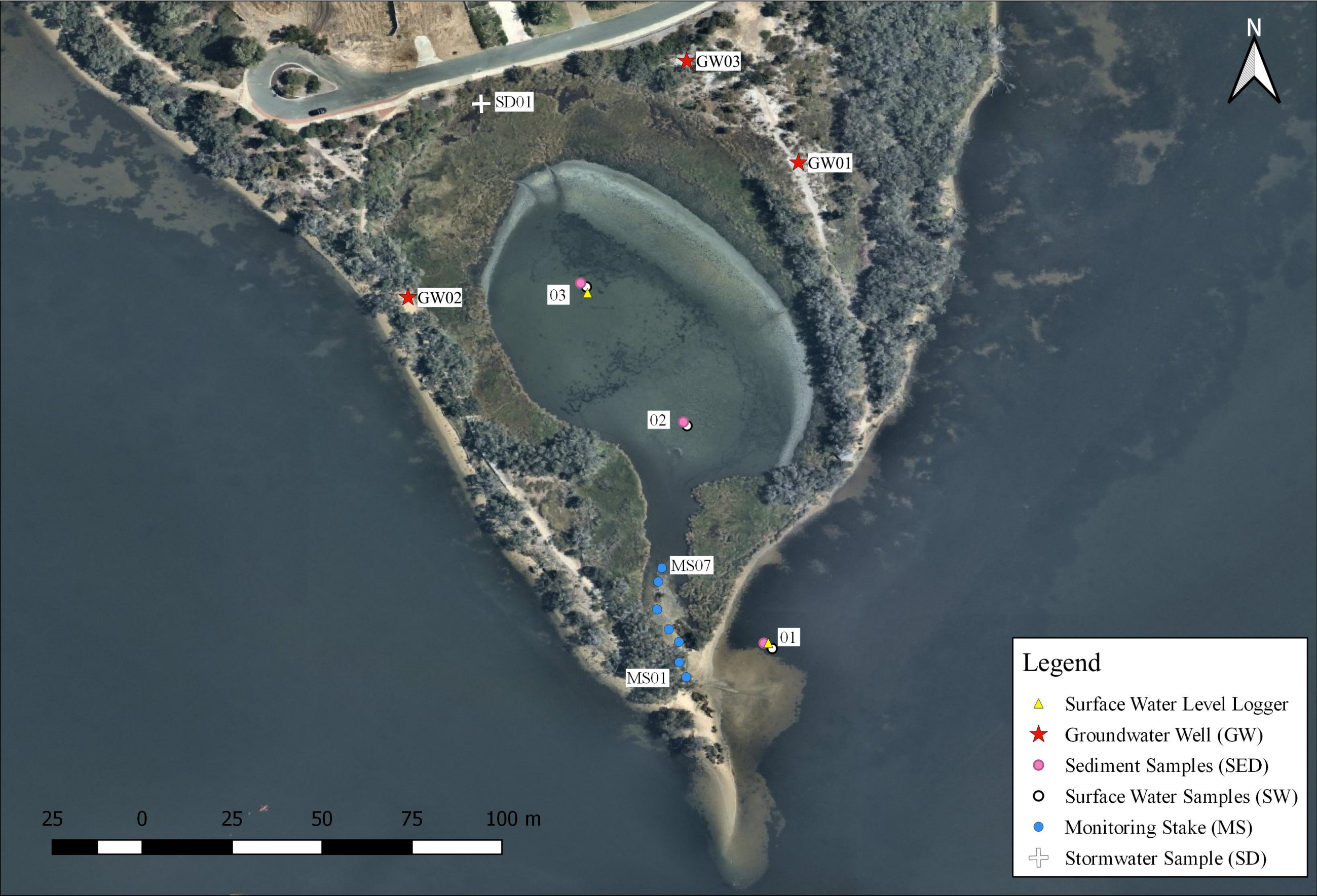
Figure 5. Salter Point Lagoon monitoring locations. Points 01, 02 and 03 are surface water (SW) sampling points for phytoplankton, physico-chemical and nutrients.
