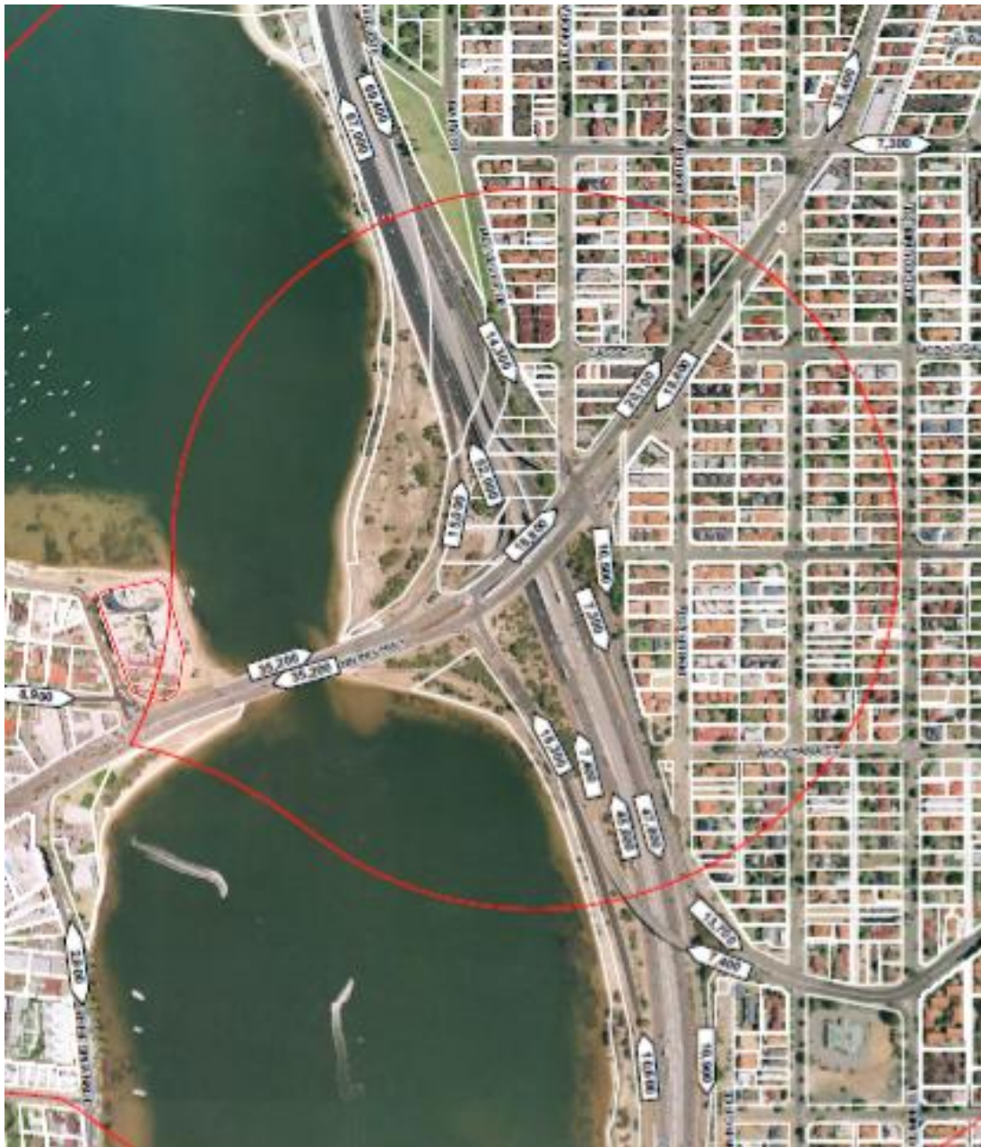
Figure 2 - Traffic volumes - Kwinana Fwy / Canning Hwy interchange
