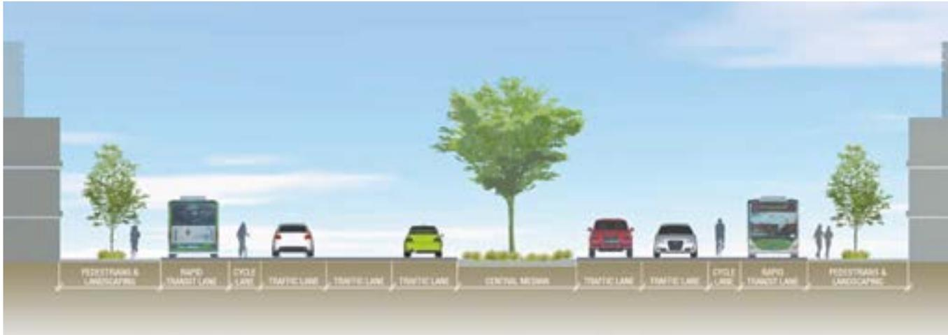
**Figure 14** Indicative cross section – Canning Highway
