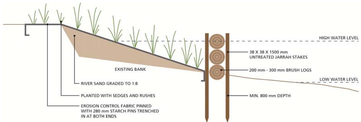
**Figure 18 Example of brush wall in front of re-graded bank**
