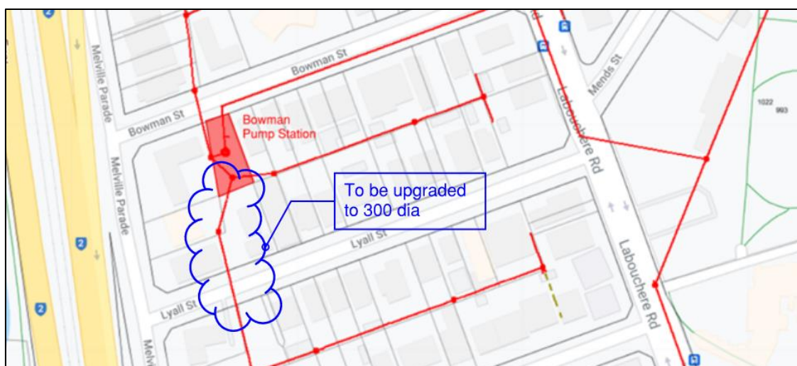
Figure 6 Bowman WWPS gravity sewer upgrade
