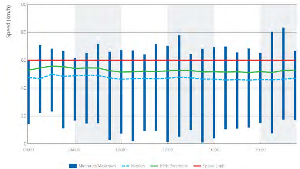
Figure 51 Speed profile Mill Point Road west of Way Road
