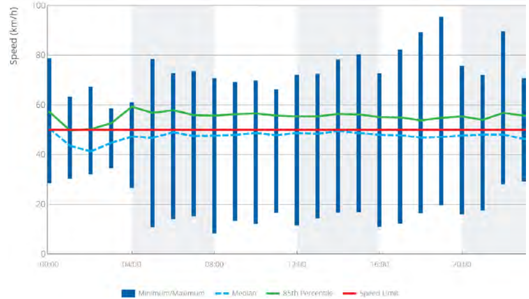
Figure 56 Speed profile Waterford Avenue south of Manning Road
