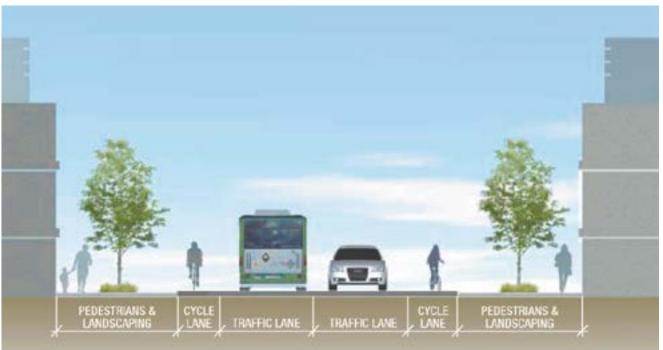
Figure 18 Indicative cross section – Local Connectors
