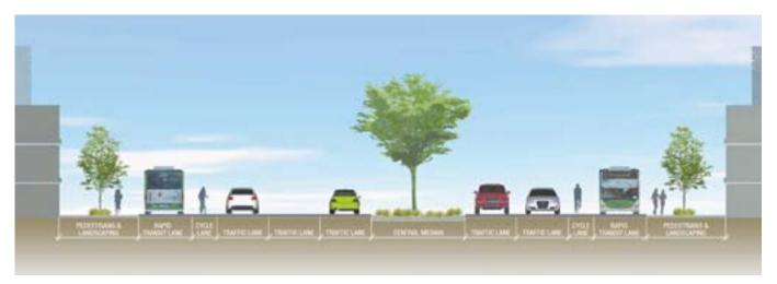
Figure 14 Indicative cross section – Canning Highway
