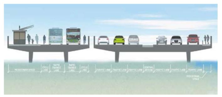
Figure 15 Indicative cross section – Canning River Bridge
