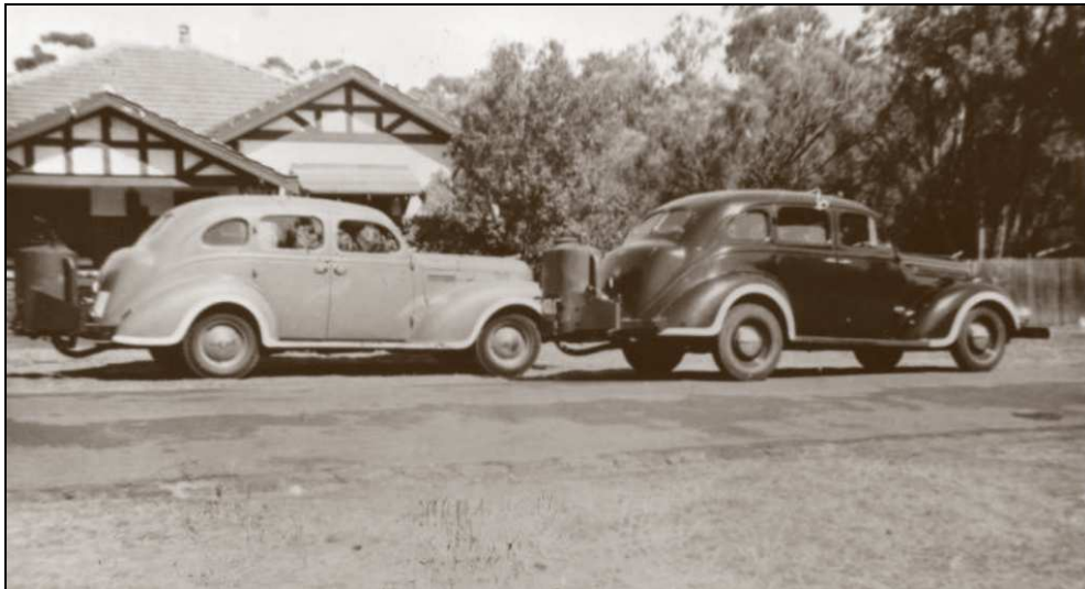
Taxis with gas converters, necessary owing to fuel shortages in World War II, 1943. (Picture South Perth Photograph Collection)
