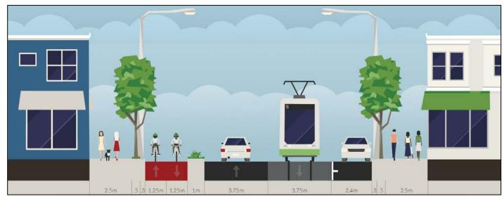
Figure 15-3: Potential Albany Highway cross section with bi-directional cycle lanes and shared light rail transit/general traffic lanes
