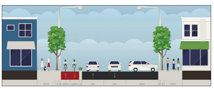
Figure 15-2: Potential Albany Highway cross section with bi-directional cycle lanes and angled parking
