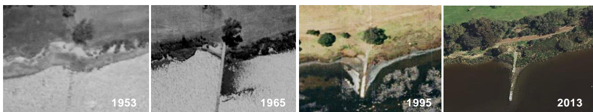
Figure 12 Changes in sand accumulation due to jetty construction (Imagery: Landgate, 2014)
